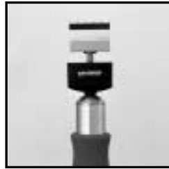
1▶ Pull down "Harris" labeled head cover from the head of the tool.
