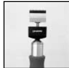
5▶ Slide cutting blade so that the blade rests completely in the head of the tool.
