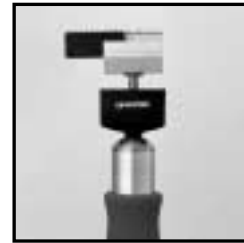
4▶ Place blade into tool with cutting blades closest to the back (jagged end) of the tool.
