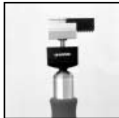
2▶ Once head cover is pulled below the head of the tool slide cutting blade out.
