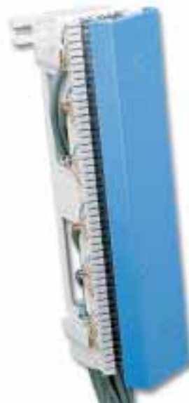
The stand-off brackets (S89D shown) allow cables to be routed behind blocks and provide a means to route cables to the front of the block for termination.
